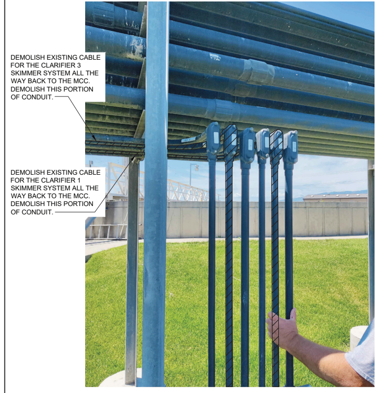
E-0003 SKIMMER CABLE DEMOLITION DETAIL SCALE: NTS
