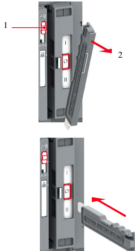
Fig. 9.2 Mounting the handle to the operating position; turn the slide switch to the Manual mode (Hand), lift the handle and place it to the operating position
