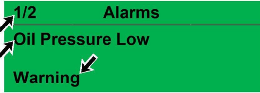
Illustration 68 g06529711 Protection Alarm
