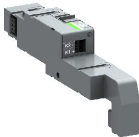
Fig. 5.7 Auxiliary power supply module, type OXEA1, is needed when Ekip Signaling, Com and Link -modules are mounted to automatic transfer switch OX_
