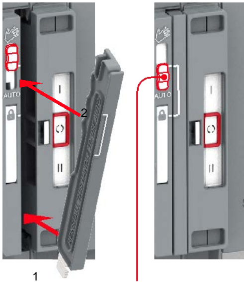
Fig. 3.6 The operating handle must returned to standby slot before moving to the automatic mode
