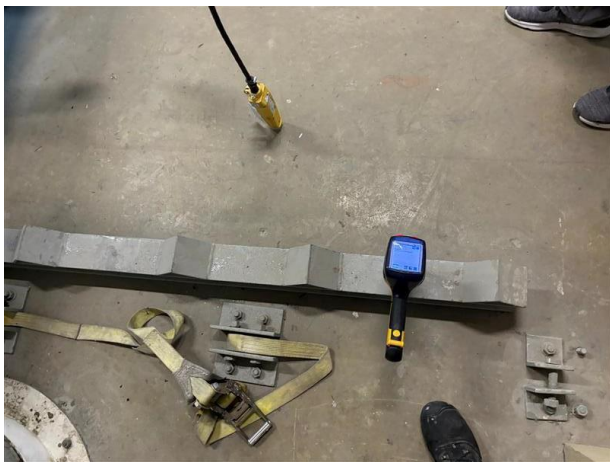
Photo #15 Chlorine storage rack—Lead concentration: 0.11 mg/cm 2
