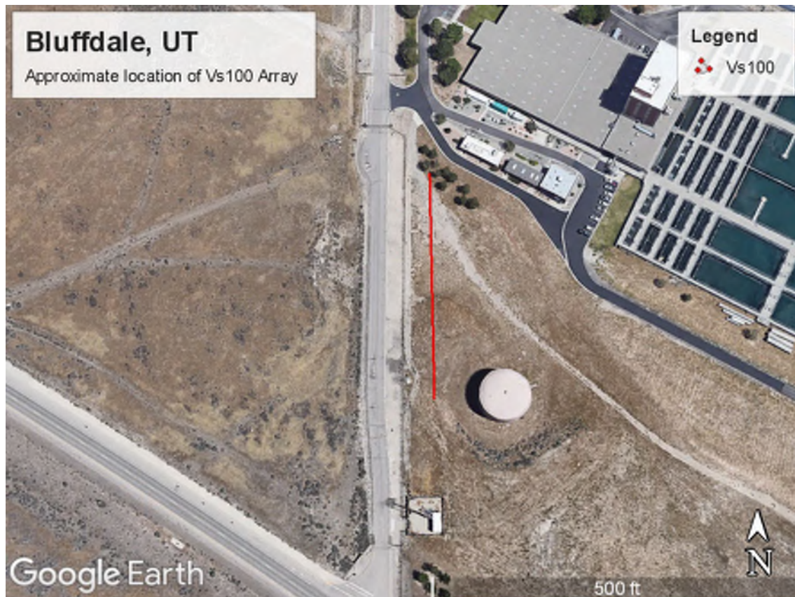
Figure 1: Shear wave velocity ( V_{s100} ) survey at the water treatment facility in Bluffdale, UT The test array length is 377 ft.
